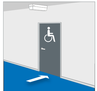
Near safe areas, for handicapped people and P.A. systems, Alarm devices in toilets for handicapped people
