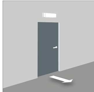
Outside the final exits and to a place of safety
