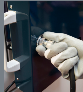
Plug in the umbilical cable
