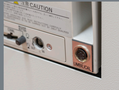
"Umbilical" socket on front cover of ACB
