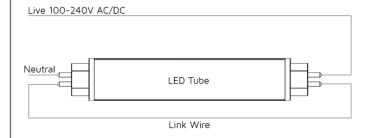
**Note:** A qualified electrican is required to remove/bypass the ballast from the fitting.
