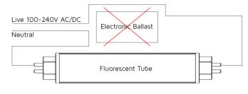
Note: A qualified electrican is required to remove/bypass the ballast from the fitting.
