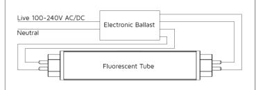
Step 2: Bypass/remove the electronic ballast along with any additional control gear or power factor correction capacitors as shown in the illustration below.
