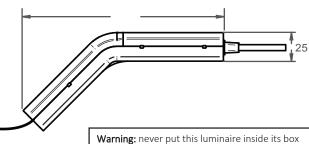
warning: never put this luminaire inside its box when it is in emergency mode. The luminaire can get damaged due to heat not being able to escape. To avoid this please disconnect and reconnect the battery before putting the luminaire back in the box.
