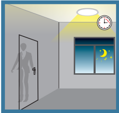
If with insufficient ambient light, the lamp dims to a stand-by dimming level (Set in the motion sensor) when no motion detected during hold time, and then switches off after stand-by period.
