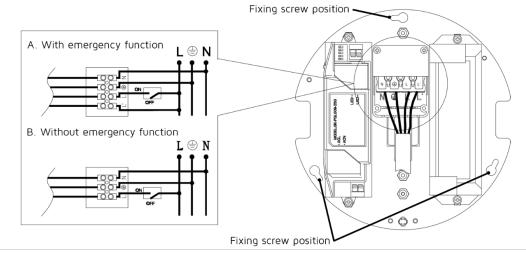
**Step 5:** Fix the cover to the body with the screws provided.
