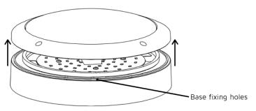
**Step 3:** Feed input power cable through a hole in the wall, then insert cable into the Bulkhead via the cable hole. Attach Bulkhead to wall with fixing screws.
