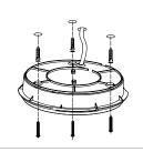
**Step 5**: Replace the diffuser by aligning it with the Gear Tray housing and rotate it clockwise. Switch on the mains supply.
