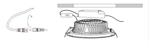
Step 3: Press clasping springs back and push downlight body into the aperture until it's fixed in the ceiling.
