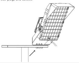
Step 3: Tilt the Sports Light to adjust it as required and tighten the bolts to lock the Sports Light in position.
