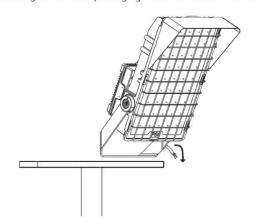
Step 2: Select a suitable mounting position and drill into the mounting surface. Screw the bracket onto the mounting surface using suitable wall plugs and screws.
