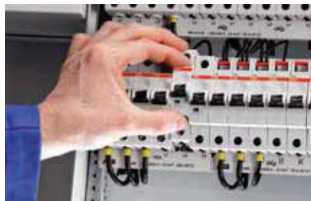
Special quick fastening for an easy removal of the devices from the assembly pressing upwards, both for MCBs S 200 and RCCBs F 200: the only in the market that can be removed without a screwdriver.
