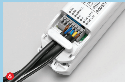
6 Connect the mains cable to the emergency LED driver (neutral conductor and unswitched line) and fix the cables with the strain relief.
