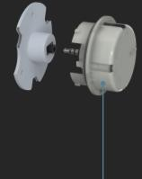
Robust die-cast aluminium housing / heatsink provides high IK08 impact rating along with optimum LED thermal management Enhancing heat dissipation away from the LED array ensuring maximum product lifetime Silicone gasket provides IP65 ingress protection
