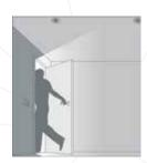
Upon entering a room the person switches on the light as normal, but on leaving the detector switches off the lighting automatically. Lights can also be switched off manually
