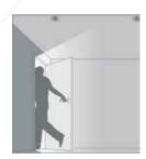
Detectors will switch on lighting automatically when a person enters the room and switches off lighting automatically when no movement is detected
