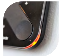
Corner illumination indicates which preset button is active
