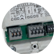
Terminals and dip-switch selection
