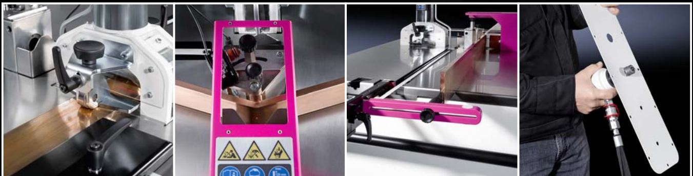
Cutting busbars to length with integral precision laser
