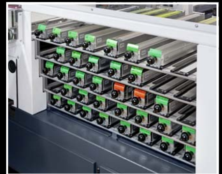
Stocking of up to 80 magazines for terminal blocks, miniature fuse-breakers etc.
