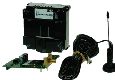
I3-MA GSM Modem with Antenna
