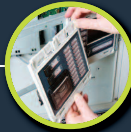
Fully interchangeable indicator modules
