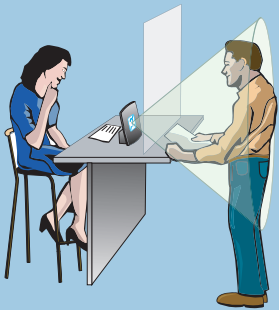
Typical counter loop system using a PL1/K1 portable hearing loop kit
