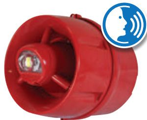
BF447C/CC/DR/65 ACTIV WEATHERPROOF W-2.75-9 WALL VAD c/w VOICE SOUNDER (IP55)
