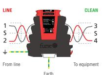
ESP RS485Q installed in series (in-line)
