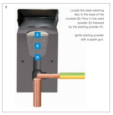
Making a FurseWELD joint is a simple procedure
