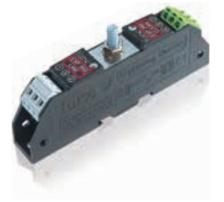
Combined Category D, C, B tested protector (to BS EN 61643) suitable for most twisted pair signalling applications. Available for working voltages of up to 6, 15, 30, 50 and 110 Volts. ESP TN suitable for Broadband, POTS, dial-up, T1/E1, lease line and \*DSL telephone applications. For use at boundaries up to LPZ 0 to protect against flashover (typically the service entrance location) through to LPZ 3 to protect sensitive electronic equipment.
