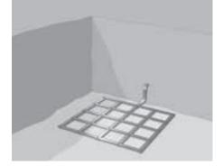
Manufactured from high conductivity copper tape, lattice earth mats are designed to minimize the danger of exposure to high step and touch voltages to operators in situations such as High Voltage switching
