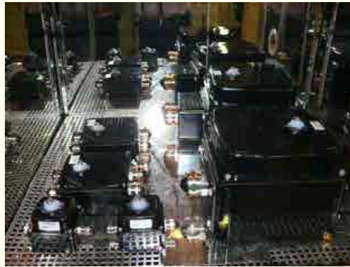
Picture 21: example of conditioning in climatic chamber
