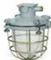
UNAV 2139 large light fixture in marine grey painted brass with stainless steel protective cage with UNAV 1948 cable gland 230V IP66
