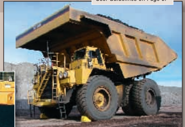
Caterpillar 793 Haul Truck (240 ton) chocked using two Model 1911 Monster Wheel Chocks.
