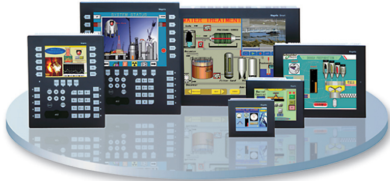
Touch screen terminals with monochrome or colour screen in 6 sizes from 3.8" to 15"
