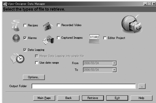
Data Manager: Transfer recipes, videos, images, etc. via Ethernet or USB, simply by clicking the mouse
