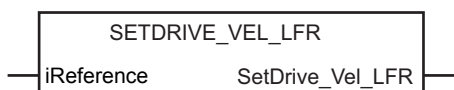
Example of a function block: sending the speed reference to the drive.
