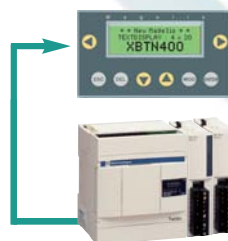
Twido programmable controller
