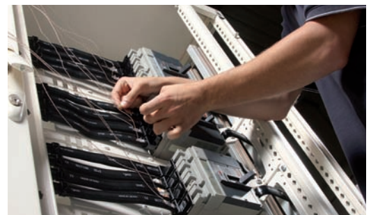
Temperature rise test in laboratory.
