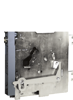
Door interlock (inhibits door opening with breaker in connected position)
