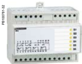
M6C programmable contacts: circuit-breaker external relay with six independent changeover contacts controlled from the circuit breaker via a three-wire connection. (maximum length is 10 meters).
