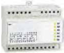
M6C programmable contacts: circuit breaker external relay with six independent changeover contacts controlled from the circuit breaker via a three-wire connection (maximum length is 10 meters).
