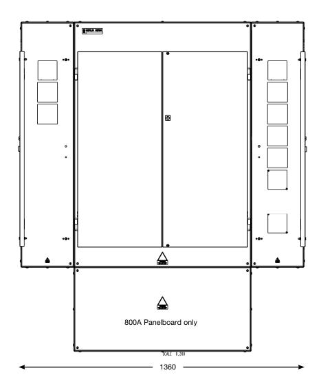
The side extensions with metering are dimensionally the same as standard 250mm side extensions
