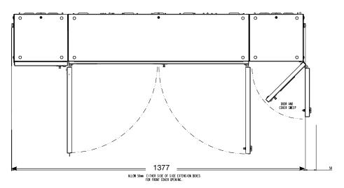
All apertures are 92mmsq. to accept standard DIN 96 meters.
