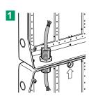
Add-on possibility Enclosures can be horizontally or vertically associated keeping the IP65 and allowing cable insertion.
