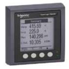
The PowerLogic PM5000 series power meter offers all the measurement capabilities required to monitor an electrical installation in a single 96 x 96 mm unit extending only 72 mm behind the mounting surface. With its large display, you can monitor all three phases and neutral at the same time. The anti-glare display features large 11 mm high characters and powerful backlighting for easy reading even in extreme lighting conditions and viewing angles.
