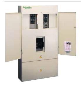
The range of wall and floor mounted Powerpact 4 panelboards is designed, manufactured and tested to BS EN 61439-1. The structures are rigid sheet steel finished in a cream colour epoxy powder (RAL 9001).
