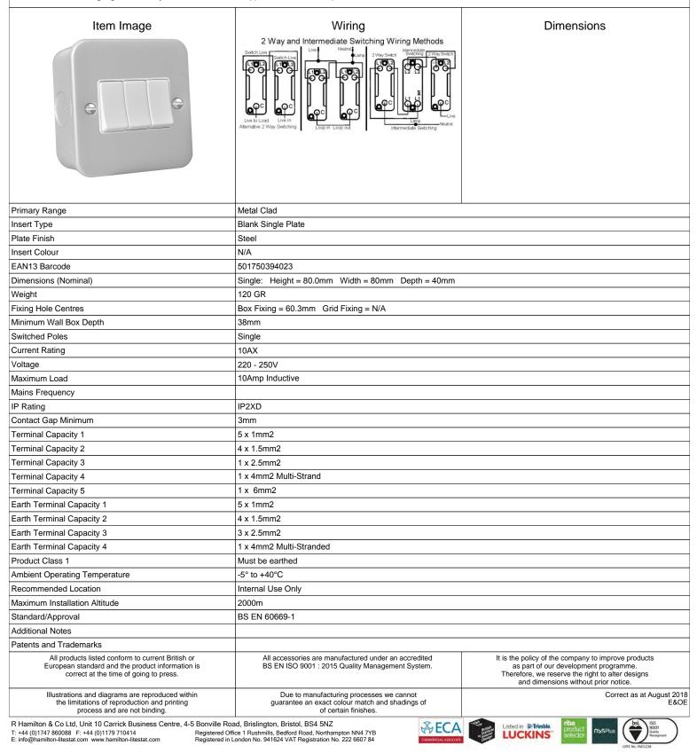
MCR23WH-W - Metal Clad Steel 3 gang 10AX 2 Way Rocker White/White supplied with 40mm Deep Metal Clad Wall Box. Wall Box includes 5x 20mm knock outs to connect to suitable conduit.
