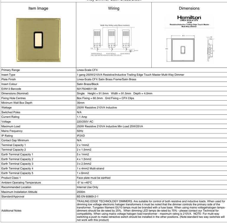
LSX1XTMSB-SBB - Linea-Scala CFX Satin Brass Frame/Satin Brass Front 1x250W/210VA Resistive/Inductive Trailing Edge Touch Master Multi-Way Dimmer Satin Brass/Black
