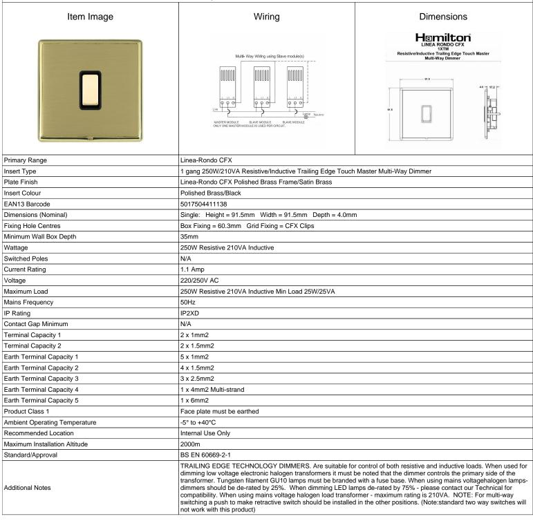
LRX1XTMPB-SBB - Linea-Rondo CFX Polished Brass Frame/Satin Brass Front 1x250W/210VA Resistive/Inductive Trailing Edge Touch Master Multi-Way Dimmer Polished Brass/Black
