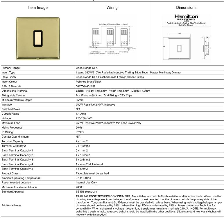
LRX1XTMPB-PBB - Linea-Rondo CFX Polished Brass Frame/Polished Brass Front 1x250W/210VA Resistive/Inductive Trailing Edge Touch Master Multi-Way Dimmer Polished Brass/Black
