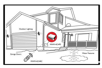
MWM-4CHPS is a mains powered radio receiver, it has four channels that will switch on/off devices such as; multiple lighting circuits, garage doors and water feature pumps. Be in control with an IR remote and have the ability to turn on lights and open the garage on approach to the property.
