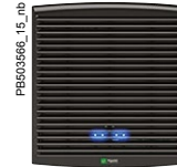
PING function Identification of the sensor on the panel (flashing blue color)
