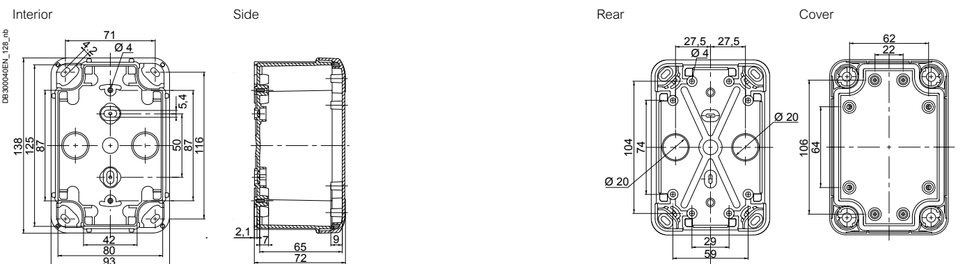
Box of 138 x 93 x 72 mm (external dimensions) NSYTB●●●1397
