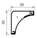
$1 = 837 \text{mm}^2 \text{ total area}$  $1 = 376 \text{mm}^2 45\% \text{ space factor}$
