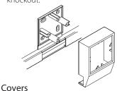
Covers are designed to limit unauthorised removal and to remain in position during normal conditions irrespective of impact and minor undulations of the mounting surface.
