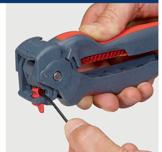
Insert cable and crimp
