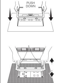
FOR SAFETY: All cables exiting boxes must be positioned into the cable routers on box trim and exit box via cable outlets
