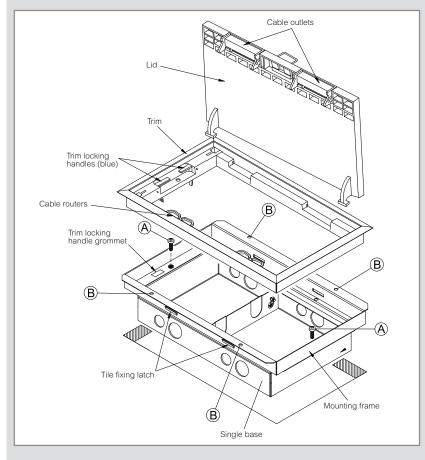
Opening lid to an angle of 30° and lifting upwards will detach lid from trim. Inserting lid into the opposite side of trim will change direction of the lid
