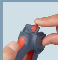
Adjust cable size
