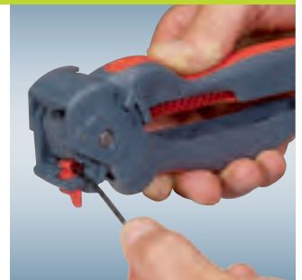
Insert cable and crimp
