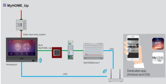
Hometouch can be used as an internal unit for video door entry systems and a touch screen for the MyHOME\_Up system Note: Hometouch connection to network can be done via LAN or WiFi
