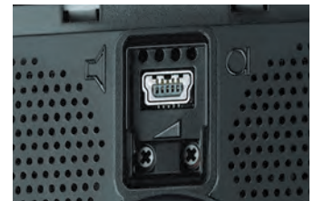
Mini-USB connection and loudspeaker/microphone volume adjustment
