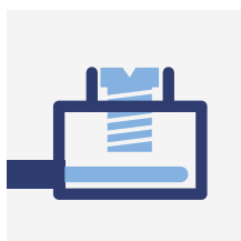
Loose screwed connections
